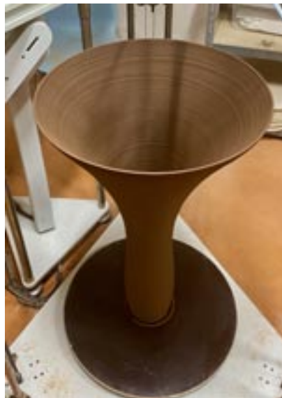
Simple ceramic pavilion 3D printed (2022) H: 85cm / gD: 50cm / pD:12cm long string acoustic amplifier on membrane (sound device in progress)
